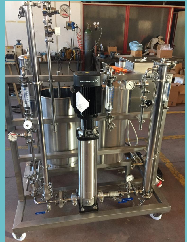
MEMBRANES PURIFICATION UNITS (micro, ultra, nano filtration and reverse osmosis)
